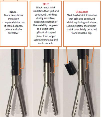
The heat-shrink tube remains in one piece but gives the appearance that a longitudinal portion is missing. This is because after splitting it shrinks in size to expose a portion of the metal tip (see picture below). If a split occurs, the heat-shrink could detach from the device before or during surgery and, if cautery is needed, there is the potential for burn due to insulation failure.
