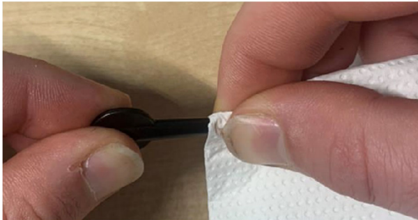
Fig. 7 – Position of the fiber cloth when holding the LDPE tube (852652)
