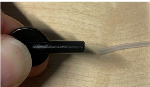
Fig. 12 - Pulling out the LDPE tube
