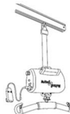
Method 2: Q-link (strap) mounted on the S65 Carriage
