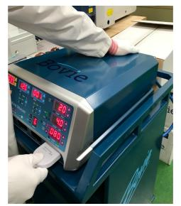
STEP FOUR - Align edge of rectangular indentation on plug with edge of generator receptacle as pictured.
