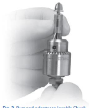
Fig. 2 Burr and adapter in Jacob's Chuck
