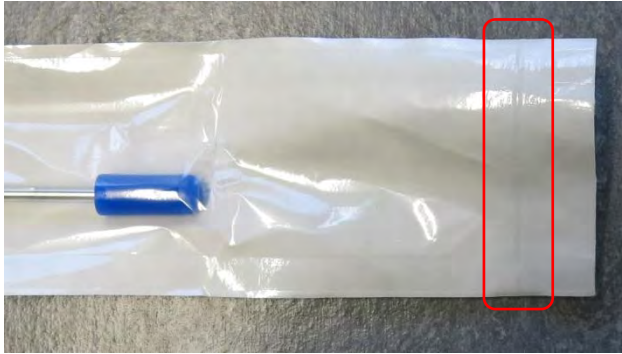
Example of sterile pouch with potentially non-conforming seal
