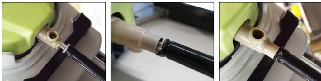
Figure 2. Examples of breaks at the roll gear and instrument shaft junction
